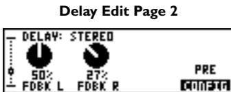
**CONFIG**, on page 2, is available for PODXT's volume pedal, Delay, and Mod. It lets you position each one either:
