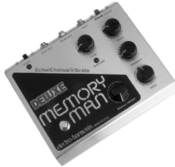
Here's a model based on the Electro-Harmonix Deluxe Memory Man which is a pedal that uses the “bucket brigade” electronics of other analog echoes, and adds a chorus circuit to boot. This adjustable chorus is applied to the echoes only, leaving the direct sound unaffected.
