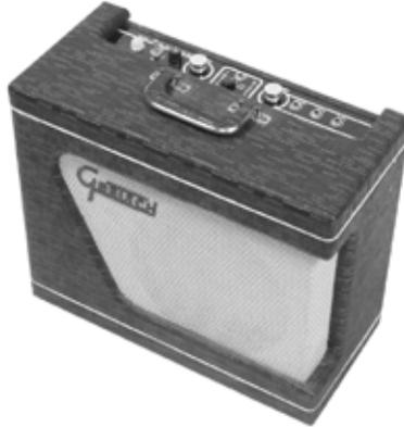
Another amp made by Valco/Supro, this is the Gretsch 6156. One of its curiosities is that the output transformer is actually mounted on its single 10-inch speaker, rather than on the amp chassis. It also has a lovely wraparound grill cloth, for a real futuristic look (or what passed for it in the '50s).
