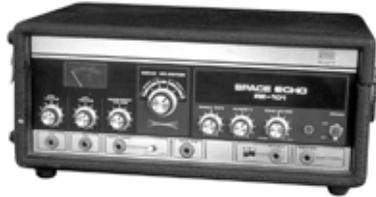
Long before Boss pedals, the RE-101 Space Echo was Roland's first venture into the world of effects processing. Instead of having one movable playback head (like the Echoplex) this machine has multiple stationary heads. You change delay times by switching amongst these heads, and then fine-tune delay time with a motor speed control. The groovy part is that you can play back on multiple heads at the same time to get multi-tap delay effects.
