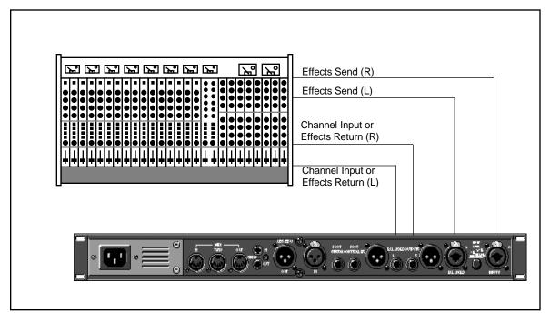
If you will be using a PCM 81 as your primary effects unit, and your system includes a console with one or more auxiliary (effects) sends, connect the PCM 81 as shown above. In most applications, it is preferable to connect the PCM 81 outputs to two of the console's input channel strips, panned full left and right, rather than to the effects returns. This allows the greatest flexibility in routing and equalization.
