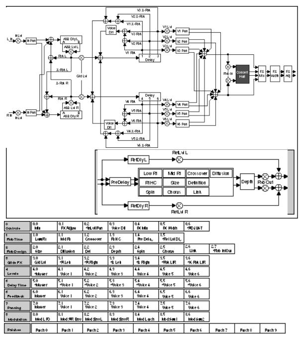
**Chorus+Rvb** The Chorus effect has six separately adjustable voices — allowing the PCM 81 to sound like a rack of six digital delay boxes. Each voice has its own independently adjustable chorus depth and rate, level control, delay time, feedback and panning control. The 6-voice chorus is in parallel with a plate algorithm, providing two independent stereo effects.
