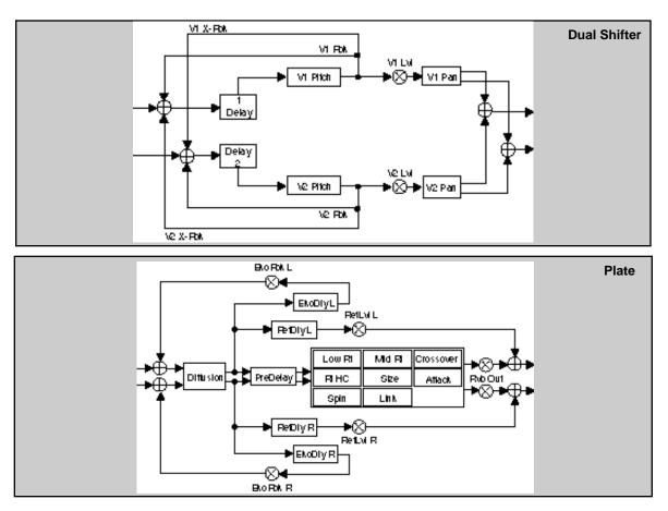
The Plate reverb mimics the sound of metal plates, with high initial diffusion and a relatively bright sound, making it a good choice for enhancing any type of percussion.
