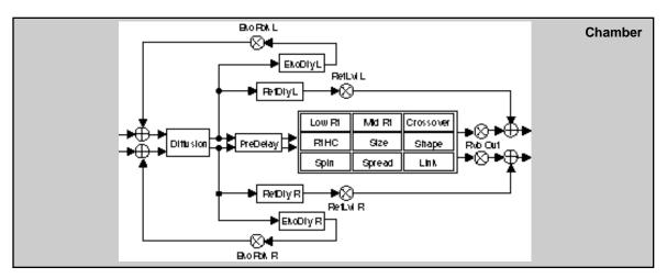
The Chamber reverb produces an even, relatively dimensionless reverberation, with little change in color as the sound decays. The initial diffusion is similar to the Concert Hall algorithm, but the sense of space and size is much less obvious. This characteristic, along with the low color in the decay tail, makes Chamber useful on a wide range of material. It is especially useful on spoken voice, giving a noticeable increase in loudness with very low coloration.
