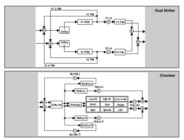
The Chamber reverb produces an even, relatively dimensionless reverberation, with little change in color as the sound decays. The initial diffusion is similar to the Concert Hall algorithm, but the sense of space and size is much less obvious. This characteristic, along with the low color in the decay tail, makes Chamber useful on a wide range of material. It is especially useful on spoken voice, giving a noticeable increase in loudness with very low coloration.
