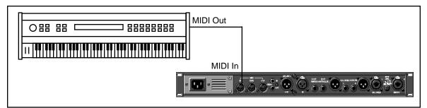
Some extremely useful effects can be created by controlling PCM 81 parameters remotely in real time. Almost all of the controllers found on a MIDI keyboard or MIDI foot controller (pitch benders, mod wheels, sliders, switches, breath controllers, foot pedals and footswitches) can be used to adjust PCM 81 parameters. We refer to this real time remote control capability as Dynamic MIDI<sup>®</sup>
