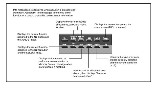
Control Mode Selections of various system states and conditions are made in Control Mode. Press Control to enter this mode. The Control button LED will light to indicate that the mode is active. Note that Control Mode functions are not available when the **Compare** function is active.
