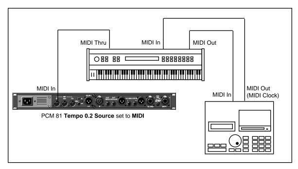
Two PCM 81s can be slaved together by connecting a cable from the MIDI OUT jack of the master to the MIDI IN jack of the slave. Additional PCM 81s can be slaved to the master by connecting a cable from the MIDI THRU port of one slave unit to the MIDI IN port of the next unit. All of the PCM 81s must be set to the same MIDI channel.
