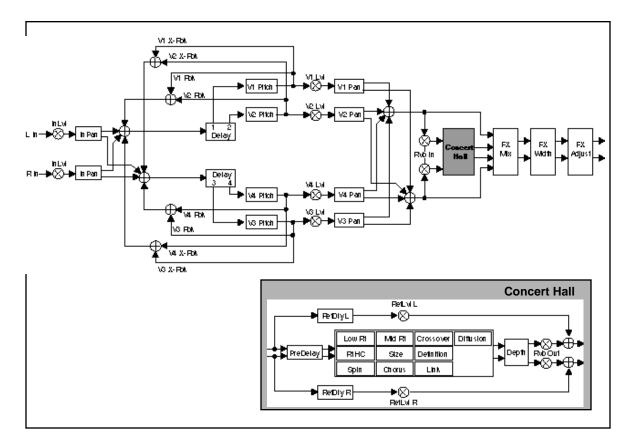
The PCM 81 Concert Hall provides very clean reverberation. It is designed to remain behind the direct sound — adding ambience, but leaving the source unchanged. This effect has a relatively low initial echo density which builds up gradually over time.
