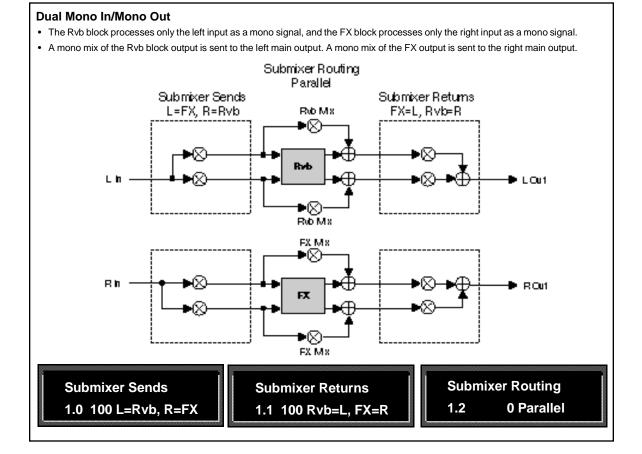
The Rvb and FX blocks shown in the previous configurations represent the Stereo Reverb and 2-Voice Pitch Shift effects. Each of these blocks has its own set of controls, shown in the diagrams below.
