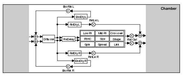
The Chamber reverb produces an even, relatively dimensionless reverberation, with little change in color as the sound decays. The initial diffusion is similar to the Concert Hall algorithm, but the sense of space and size is much less obvious. This characteristic, along with the low color in the decay tail, makes Chamber useful on a wide range of material. It is especially useful on spoken voice, giving a noticeable increase in loudness with very low coloration.
