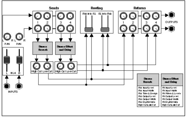
The Dual-Chmb, Dual-Plt, Dual-Inv and Stereo-Chmb algorithms contain a complete dual-channel effects mixer. The Submixer appears as row 1 on the parameter matrix. The first three parameters in the row are the basic Submixer controls: Sends, Returns, and Routing. Any configuration can be achieved by simply adjusting these three parameters.
