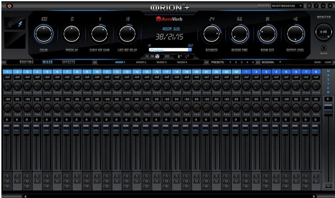
The Mixer tab is home to four 32-channel software mixers. Each channel is equipped with Pan, Volume, Solo, and Link controls (on odd-numbered channels), as well as metering. The Master channel has Volume and Mute controls.
