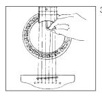
Clockwise rotation of the tension rod adjustment will tighten the tension rod to correct a warped condition. Use the previously outlined procedure to check your adjustment. Make sure that you do not overtighten the tension rod and lose the clearance at the 5th fret.
