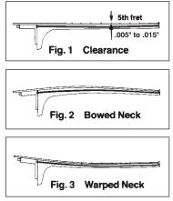
2. Check the clearance between the bottom of the string and the top of the 5th fret.
