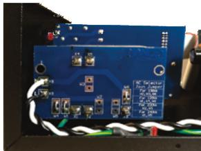
*The Type 2 SMPS MANLEY POWER® power supply will work everywhere on earth. It does not need to be reconfigured for different countries' mains voltages (90-250VAC) and will operate on any mains frequency (50 or 60 Hz).*
