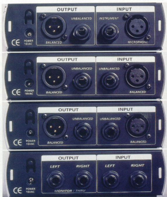
The rear panels of the four units in the range (top to bottom): Tube Pre, Comp16, EQ3B, and HP4.
