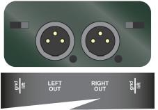
NOTE: DESCIPTIONS FOR THE FOLLOWING ARE IDENTICAL FOR THE LEFT AND RIGHT OUTPUTS.
