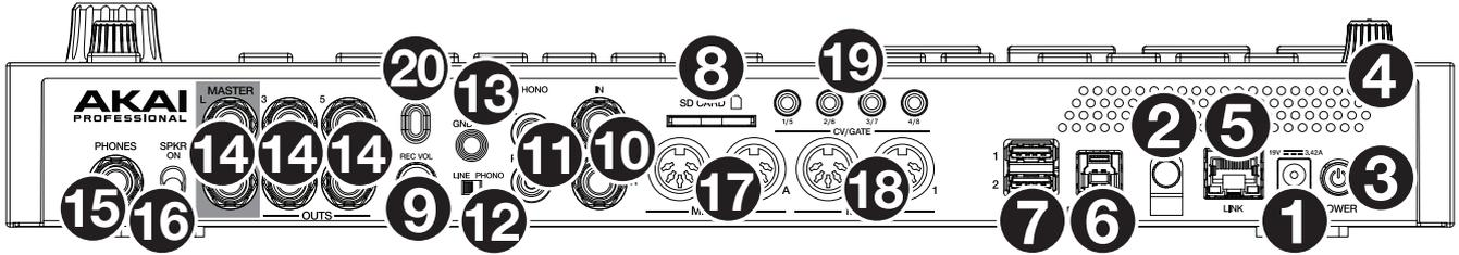
1. **Power Input:** Use the included power adapter to connect MPC Live II to a power outlet.
