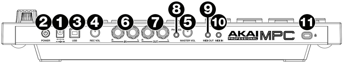
1. **Power Input:** Use the included power adapter to connect MPC Touch to a power outlet. Alternatively, you can power MPC Touch via the USB port only, but the touchscreen will be disabled.
