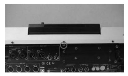
5. Use both hands to lift the protrusion on the front of the top panel, and open the top panel.
