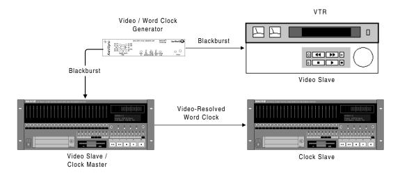
One can also distribute word clock to all the digital audio devices from an external source (such as the Aardsync II from Aardvark depicted above) that generates both a master video blackburst and a resolved word clock output.
