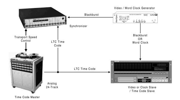
It is important to note that MTC should not be used when resolving sample clock to time code; LTC is the preferred choice. This is because the LTC signal has much greater timing resolution than MTC.
