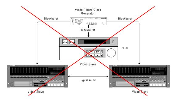
When digital audio signals are connected between digital audio devices it is imperative that their clocks be synchronized to a common word clock source, regardless of whether or not video synchronization is involved.
