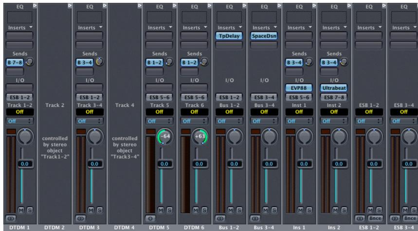
This mixer example features six Audio Track Objects, two Bus Objects, two Audio Instrument Objects, and two stereo sums. It is possible to engage up to 255 Audio Track Objects and 64 Bus Objects.
