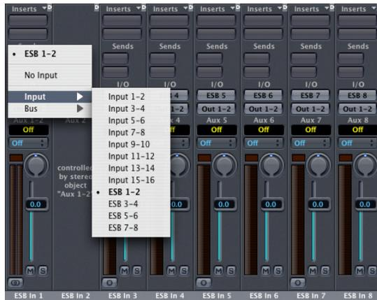
Please note that Logic handles mono and stereo channel settings separately. This means that you can set up the ESB inputs for eight mono channels, and then switch the Audio Objects to stereo operation. Once the desired DTDM output channels are set appropriately for each Aux Input, save your Autoload Template. This will allow you to switch quickly between mono and stereo setups, without needing to reset the settings each time.
