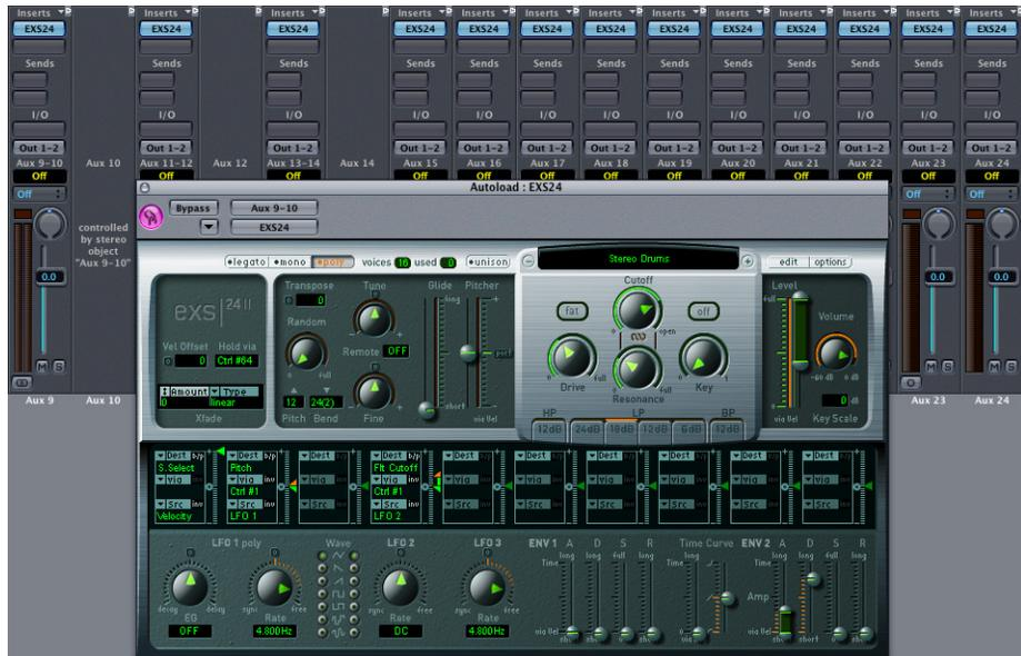
In the example shown, multiple EXS24 sampler instances have been inserted into the Aux Objects 9–24.
