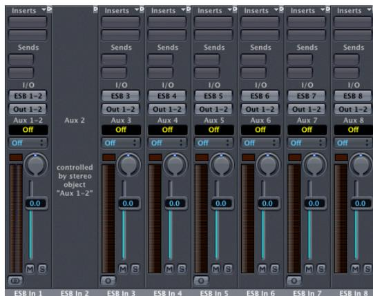
Within mono Aux Objects, you can select the desired output channel of the DTDM mixer (ESB 1–8). Stereo Aux channels can be set to input channel pairs ESB1–2, 3–4, 5–6, and 7–8. Please take a closer look at the available inputs:
