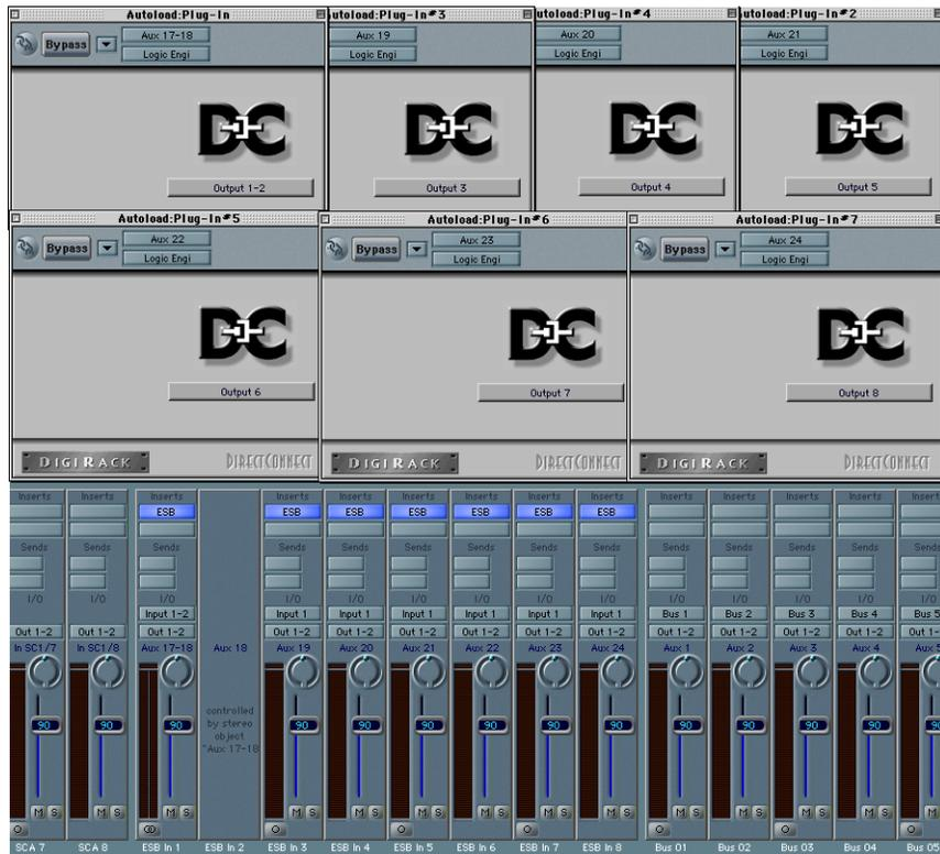
Within the ESB TDM Plug-in window, you could select the desired output channel of the DTDM mixer (Outputs 1–8). ESB TDM plug-ins inserted in stereo Aux Objects could be set to output channel pairs 1–2, 3–4, 5–6, and 7–8.
