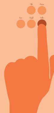
Press and hold the **Velo** button for 1 second to enable or disable velocity response. The LED will turn on when velocity is enabled and turn off when velocity is disabled.
