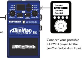
**NOTE:** All audio signals connected to the Aux input are summed to mono.
