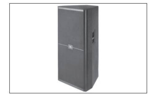
The enclosure is constructed of top quality birch plywood and coated in JBL's rugged DuraFlex<sup>™</sup> finish. The attractive CNC-machined, 16-gauge steel grille wraps around the sides of the enclosure so there are no protruding lips on the front of the box to create acoustical interference. The grilles are internally lined with acoustically transparent foam to provide additional driver protection and give a very professional appearance.
