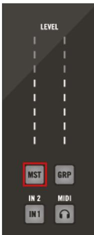
2. Turn the Encoder to adjust the level of the main volume. Hold **SHIFT** and turn the Encoder to adjust the value in finer increments.
