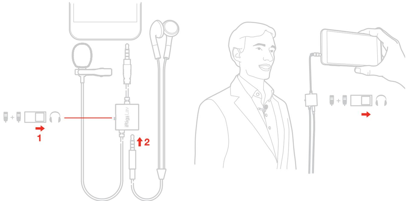
Thanks to the female 1/8" TRRS connector on the in-line connector it is possible to connect either a second iRig Mic Lav or a headphone.
