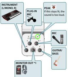
(\*1) The [MONITOR OUT] knob adjusts the overall volume that is recorded.
