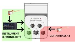
(\*3) If you're routing your guitar (or bass) through an effect device, connect it to the INSTRUMENT jacks.
