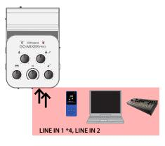
\*4) Sound from a device connected to the LINE IN 1 jack can be used for karaoke (p. 19).
