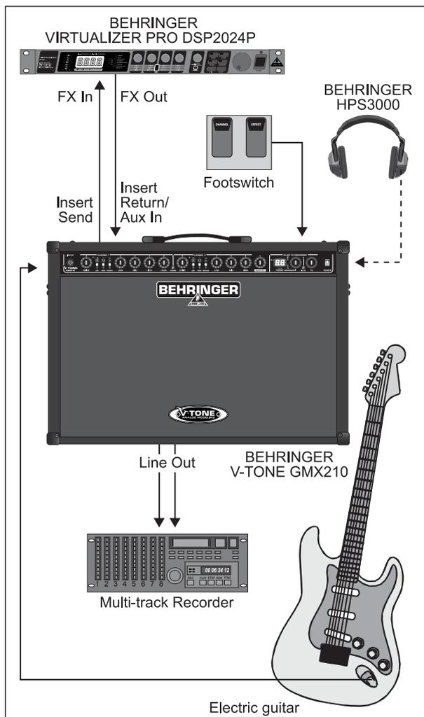
Fig. 3.2: Recording setup
