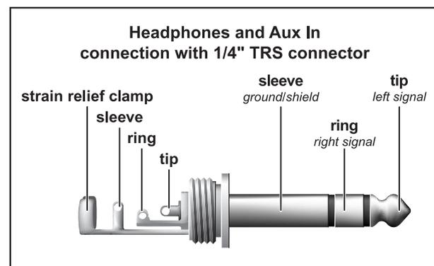
Fig. 6.2: 1/4" stereo TRS connector for AUX and PHONES
