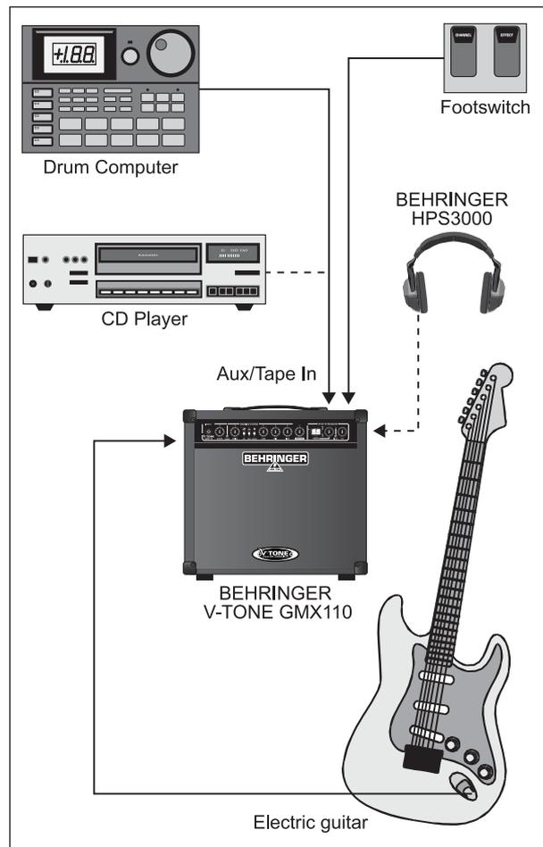
Fig. 3.1: Standard setup
