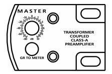
**MASTER (LEVEL):** This control adjusts the output level of the EUREKA. It functions as a master fader for the entire processing strip. It is useful for adjusting the overall output level up or down to match the optimum input level of a recorder, mixer, etc.
