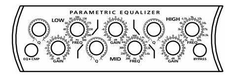
The EQ is divided into three sections or bands (Low, Mid and High) Each band has the following controls:
