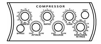
**THRESHOLD:** Sets the level at which compression begins. The below and above LED's over the Threshold knob indicate whether the input signal is below or above the Threshold setting. When the signal is above the Threshold setting, it becomes 'eligible' for compression. Basically, as you turn the Threshold knob counter-clockwise, the input signal is compressed. (If you have a ratio setting of greater than 1:1.)
