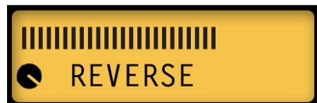
Reverb isn't in the SmartFX group, but it also features a primary and secondary model, as illustrated below. Like the SmartFX, you select the model by turning the Presets knob when the Reverb model name is displayed in the LCD. The difference is, the bar graph for Reverb indicates its Mix level, which matches the Reverb knob position when you turn it.
