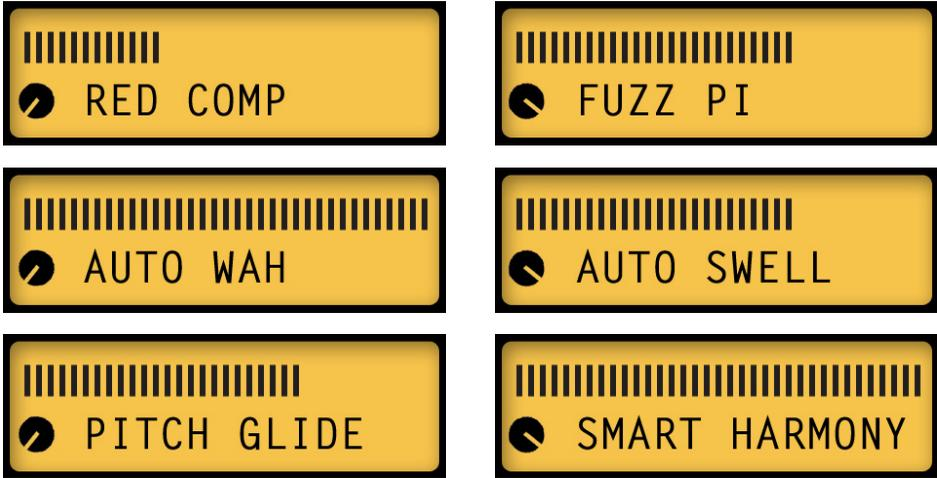
Above are the primary and secondary FX1 models for the Gain, Auto and Pitch locations. The small knob at min position indicates primary model; max position indicates secondary. The bar graph displays the selected effect's current swoosh position on the FX1 knob.
