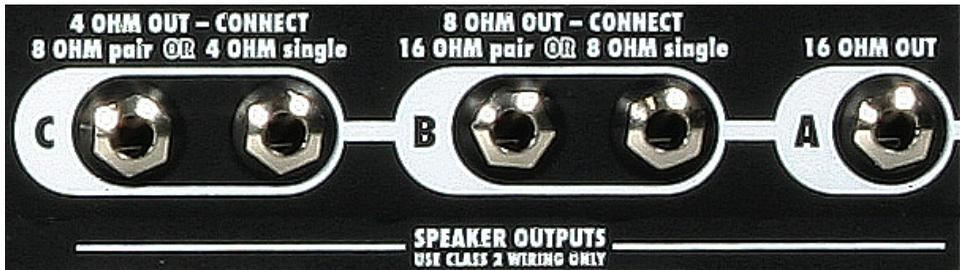
**A 16 Ohm Out** – If you’re using one 16 Ohm cab, a 4x12 for example, connect it to the single A Speaker Output.
