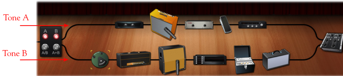
Signal Flow View - Dual Tone Mode
