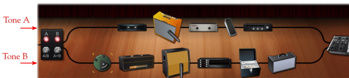
Signal Flow View - Dual Tone Mode
