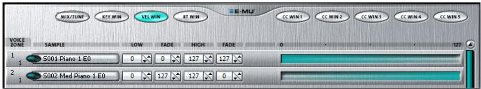
2. Select the Velocity Window tab shown above. By default both voices will be assigned to the full 0-127 velocity range.
