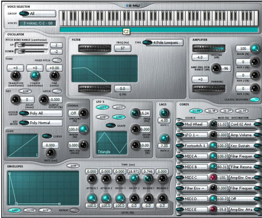
The voice editor window displays all the synthesizer controls and PatchCord routings for the selected voice(s). Each module, surrounded by the blue borders, contains an independent synthesizer function.
