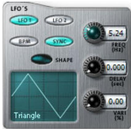
A Low Frequency Oscillator or LFO is simply a wave which repeats at a slow rate. LFOs are used to add animation to a sound. Emulator X has two multi-wave LFOs for each voice, with 17 different waveforms which are diagrammed below.
