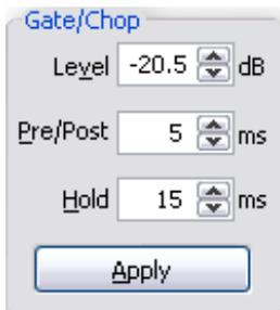
1. Set the threshold **Level** using the numeric display or by setting the threshold markers in the waveform display. This setting affects the accuracy of the gating. For percussive samples like the ones shown above, set this setting at -40 dB or lower to start. Different signals require different settings.
