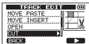
This function cuts (deletes) the audio data between the IN and OUT points on the selected track, and shifts the remaining recording after the OUT point forward to the IN point. Therefore, the track becomes shorter.
