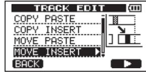
The audio data between the IN and OUT points on the MOVE source track is removed and inserted in the MOVE destination track from the TO point. This operation leaves a silence between the IN and OUT points on the MOVE source track.
