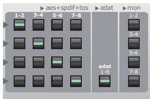
Each input channel pair can be routed to any AES/SPDIF/TOS output and to ADAT outputs.
