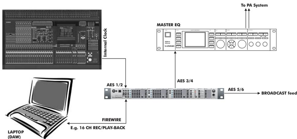
In this example Digital Konnekt x32 is used in a live situation as a digital splitter box that routes the signal to both a laptop computer for recording/play-back, to the PA system via a master EQ and to a broadcast station.
