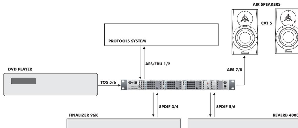
This example illustrates Digital Konnekt x32 used in conjunction with a ProTools setup integrating external digital devices. The screenshot in this example is based on ProTools HD but applies for any version of Pro Tools hardware that has digital in (AES/EBU, SPDIF, ADAT, TOS or Word Clock).
