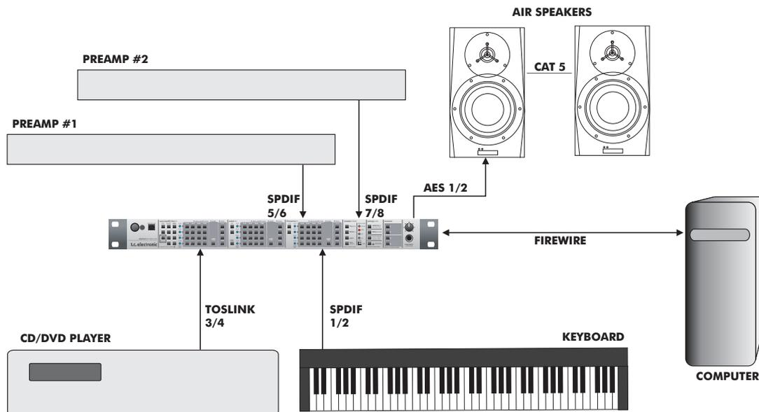
In this example we show how to use the Digital Konnekt x32 as a more conventional audio interface where four different external digital sources are connected. For monitoring we have connected a couple of Dynaudio Acoustics Air monitors equipped with the AES/EBU input option installed.
