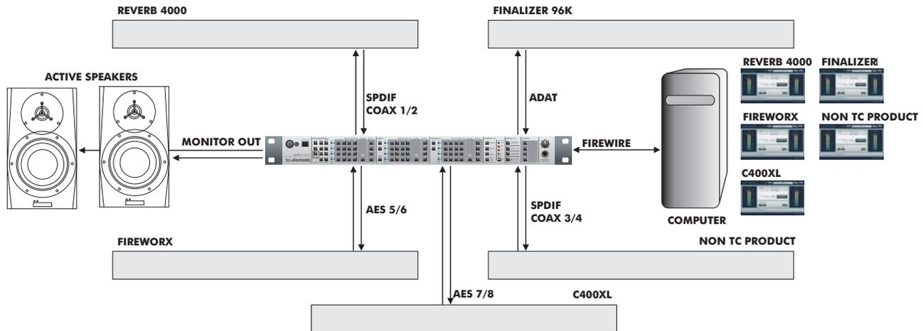
In this example we show how Digital Konnekt x32 and the Integrator plug-in allows integration of external digital effect devices with your DAW via Firewire.
