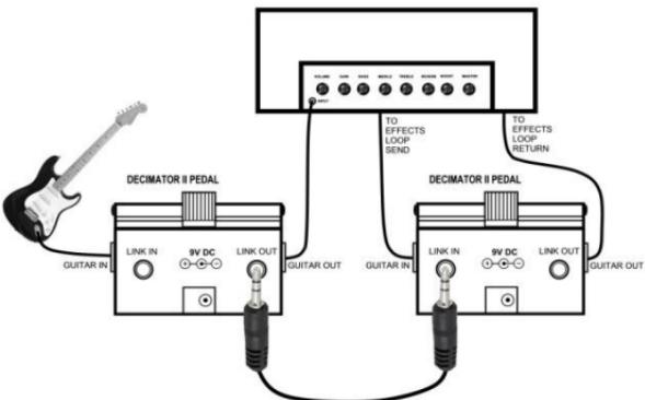
The guitar is connected to the input of the first pedal and Guitar Out feeds the input of a guitar head or input of a pedal chain. The second Decimator II is connected in the effects loop of the Head with Send connected to Guitar IN and Return connected to Guitar OUT. Adjust the Threshold by setting the Threshold of the first pedal to remove the noise of the Guitar first and then adjust the second pedal Threshold to remove the HEAD gain noise.
