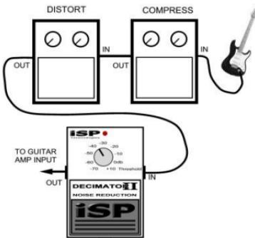
For best performance place all gain pedals in front of the Decimator II. You can put Delay and Reverb effects pedals after the Decimator II to avoid cutting off reverb and delay tails. NOTE: When connecting the Decimator into the effects loop of your amplifier connect the send to the Decimator II Input and return to Decimator II Output.
