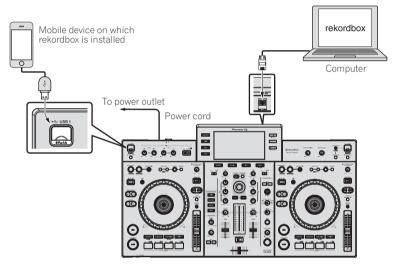
1 Connect the unit and the computer by using a LAN cable, or connect the unit and the mobile device by inserting the available USB cable in the USB device insertion slot.
