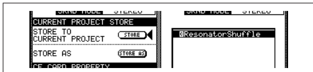
Figure 2.33: Storing a project
