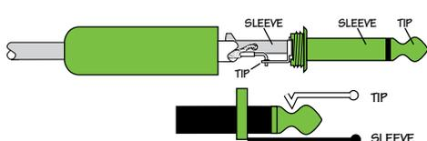
**1/4" TS Unbalanced Mono Wiring:**
