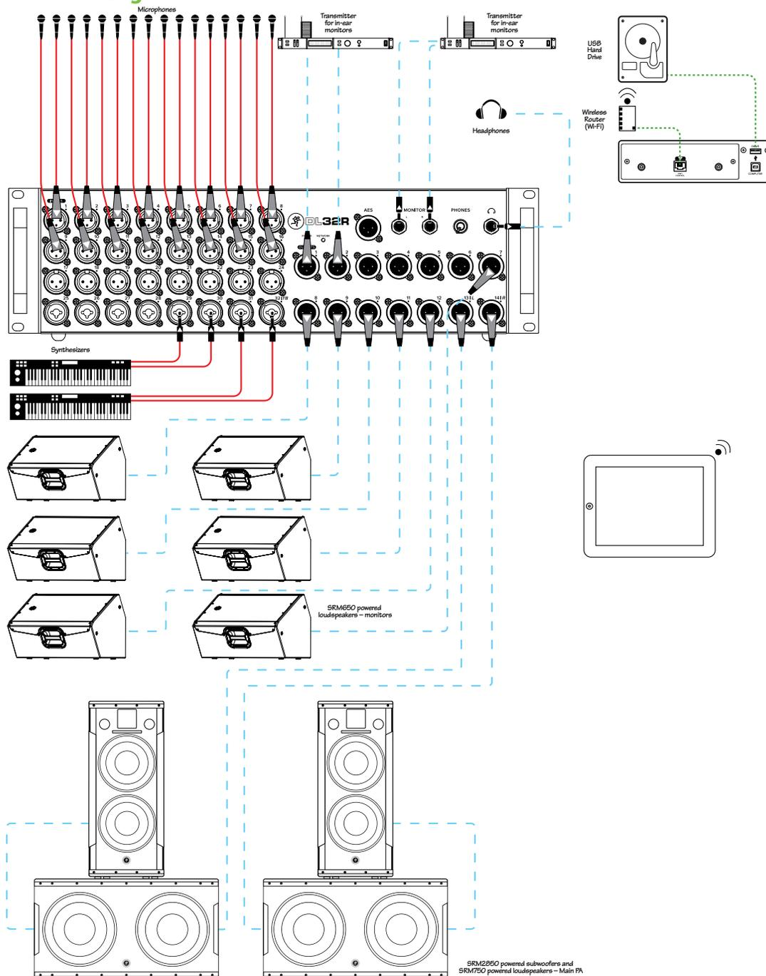
Here's a pretty common setup utilizing the DL32R. Mics are connected to input channels 1-16 which may be used to mic up a drum set, guitar and bass cabinets, acoustic guitar, lead and background vocals, a horn section, etc. A pair of synthesizers are connected to channels 29-30 and 31-32 via 1/4" input jacks. And there are still an additional 12 unused inputs available for extra mics!
