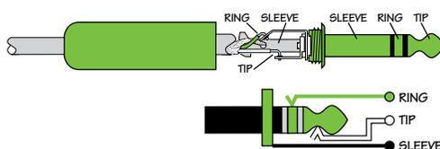
**1/4" TRS Balanced Mono Wiring:**
