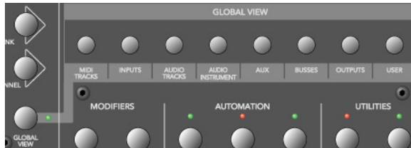
Pressing multiple GLOBAL VIEW buttons simultaneously will display the channels of the selected classes.
