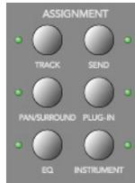
These ASSIGNMENT buttons work in both *Track* and *Global View* modes. View modes are discussed in the *Track View Mode* section, from page 17 onwards.
