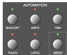
The five buttons in this area activate/deactivate the various automation modes of Logic. These work in conjunction with the channel SELECT buttons. Simply choose the channel you wish to automate, select the *Automation* mode via one of these six buttons, and move the corresponding fader. The modes are outlined below:
