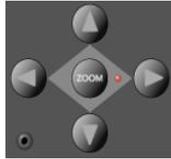
When holding down the OPTION button, the CURSOR LEFT/RIGHT buttons scroll to the first/last page, and the CURSOR UP/DOWN buttons scroll to the first/last slot.
