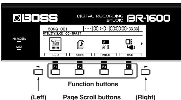
[F1] through [F4] are called the FUNCTION buttons. At the bottom of the display, you will find the names of the functions that are assigned within the current screen to each of these buttons.
