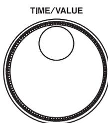
The TIME/VALUE dial is used to change the cursor position, values, or characters. In the case of values, these are increased when the dial is turned clockwise, and reduced when the dial is turned counterclockwise.
