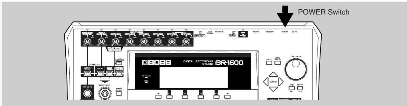
**1** Before turning on the power, the volume of all connected devices should be turned all the way down.
