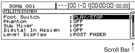
When you see a scroll bar at the right of the screen, it means that the BR-1600CD could not fit all of the relevant content in one screen, and there is additional content hidden at the top or the bottom.
