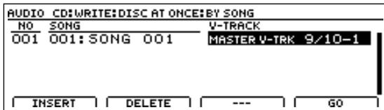
At this time, "MASTER V-TRK" will be indicated for the V-Track that was most recently used for mastering (i.e., the final mastering track). This can be used as a guide for setting the correct V-Track.
