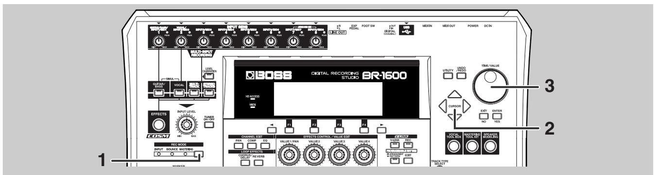
**1** Press [REC MODE] several times until the MASTERING indicator lights up.
