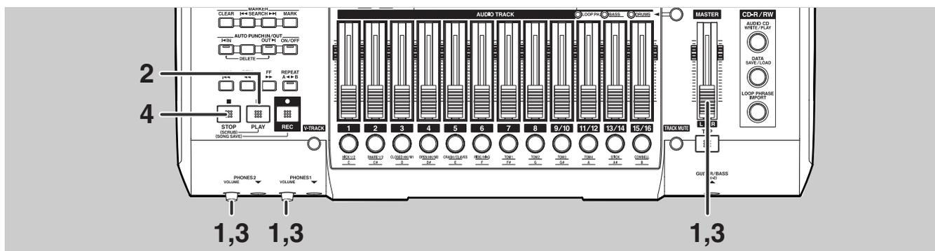
**1** In order to avoid being startled by sudden loud noises, turn the PHONES 1 & 2 VOLUME knobs and the MASTER fader all the way down before proceeding.
