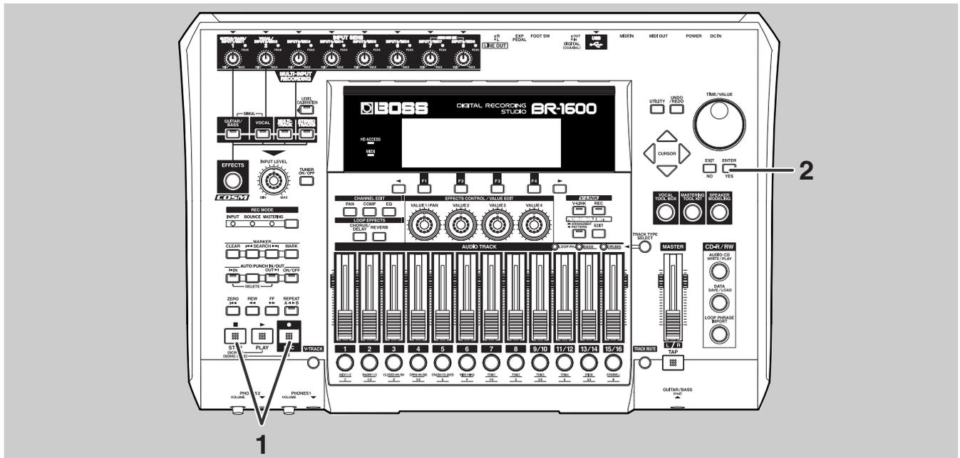
**1** With the top screen displayed, hold down [STOP] and press [REC].
