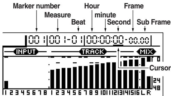
The current position within the song is indicated in terms of time at the top right of the display. In addition, this position is also indicated in terms of bars and beats to the left of this time value.
