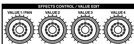
These knobs can be used to change the values of parameters indicated by knob icons (
