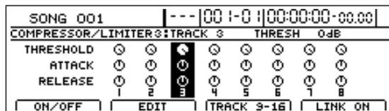
Press [F3] (TRACK 9-16) to switch to the setting screen for Track 9/10 through 15/16. To return to the setting screen for Track 1 through Track 8, press [F3] once again.
