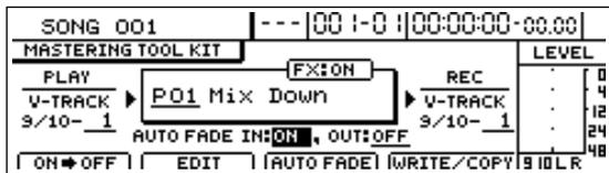
Displayed shortly after the power is turned on, this is the main BR-1600CD screen. Among other important information, the top screen presents the name of the currently selected song, the current position within the song, the level meters, and remaining recording time on the hard disk.
