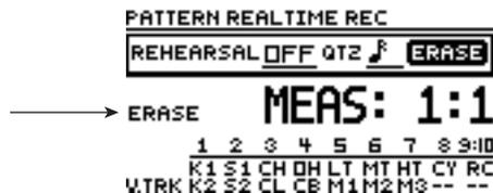
3. To erase an individual note, press and hold its TRACK button just before the note would sound and then quickly let go of the button.
