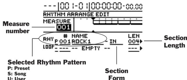
3. Let's start at the beginning with a four-bar introduction. Turn the TIME/VALUE dial to select Measure 001 if it isn't already selected. The BR-1180CD offers different versions, or "forms," of its rhythms that are specially designed for the various types of sections a song might have. Choose the desired form for the currently selected section.
