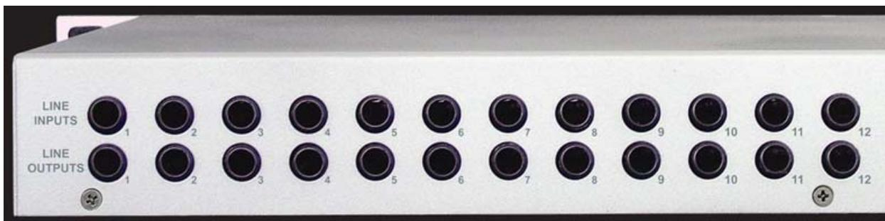
By default, the inputs and outputs are set to receive or send a +4dBu signal. You can switch between +4dBu and -10dBV for each individual input and output via the console software (see section below).
