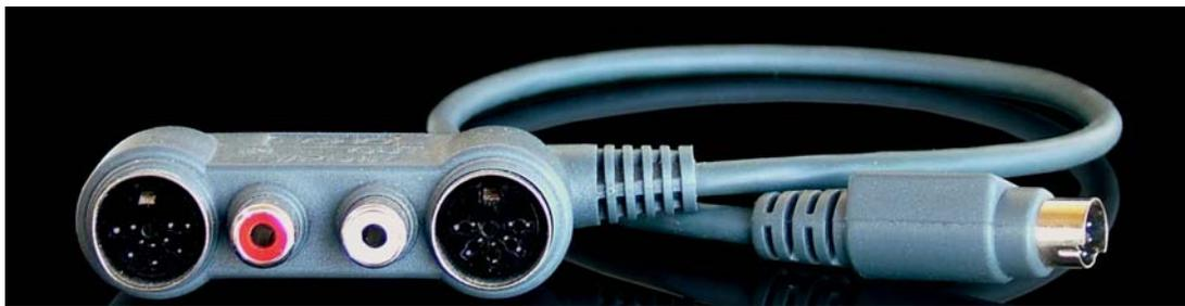
The S/PDIF connectors are used to transmit digital audio data between digital audio devices via an electrical signal. When connecting devices to the S/PDIF jacks, the use of standard analog RCA audio cables is not recommended. For reliable S/PDIF operation, 75-ohm coaxial (RG59) video cables are recommended.
