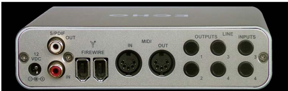
You can switch between +4dBu and –10dBV for each individual input and output via the console software (see section below).
