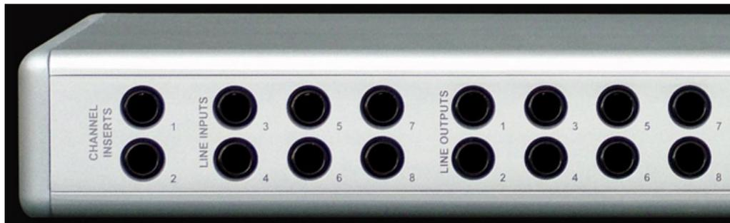
You can switch between +4dBu and –10dBV for each individual input and output via the console software (see section below). There are also two channel inserts on the rear panel where you can connect a serial effects device (compressor, EQ, etc.) for the universal inputs (1 – 2). The channel inserts are wired: tip = send, ring = return and sleeve = ground.
