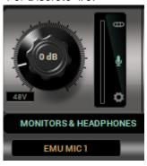
Choose EMU MIC with the corresponding channels for the mic inputs. This way you will record the processed signal with the loaded emulation. You can also choose a mix on emulated and dry preamp signal, with a combination of a couple of channels (Emu and Preamp)
