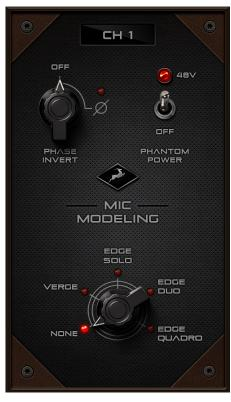
Note:48V Phantom power will be automatically enabled.
