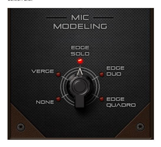
Mode switch – allows you to switch between Verge and Edge mic types or turn the emulation off.
