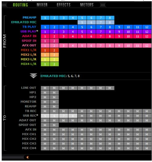
Again, you can record dry and wet signal with a combination of the Emulated mic channels and the physical input channels.
