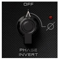
**Phase invert** – allows you to invert the polar pattern of the signal in the selected Mic input.
