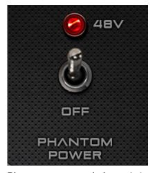
**Phantom power switch** – switched on by default, when you're loading a Mic Emulation in the AntelopeAudio interface Control Panel.
