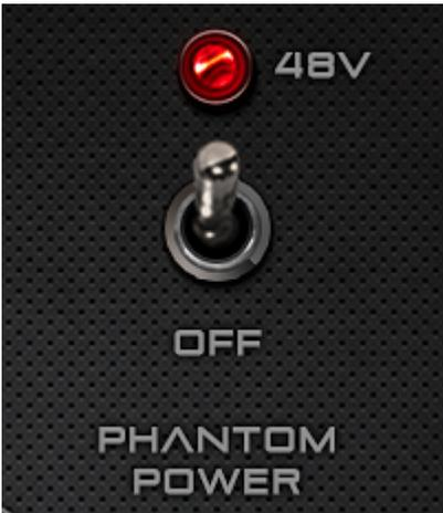
Phantom power switch – by default switched on when you're loading a Mic Emulation in the Antelope Audio interface Control Panel.
