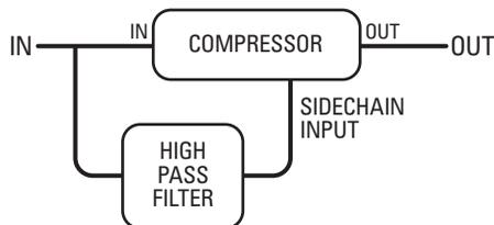
SYBIL Evo uses a digital algorithm to implement the de-esser function. While the details of the algorithm are quite complex, the resulting effect is functionally equivalent to the diagram above.
