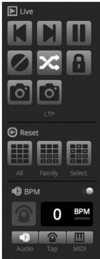
The all new Show Mode\* allows you to quickly create a custom screen and use it on a touch screen, or send it to an iPhone/iPad or Android device. Pairing commands can be done simply by holding ALT and clicking on the part of the software that you wish to link.
