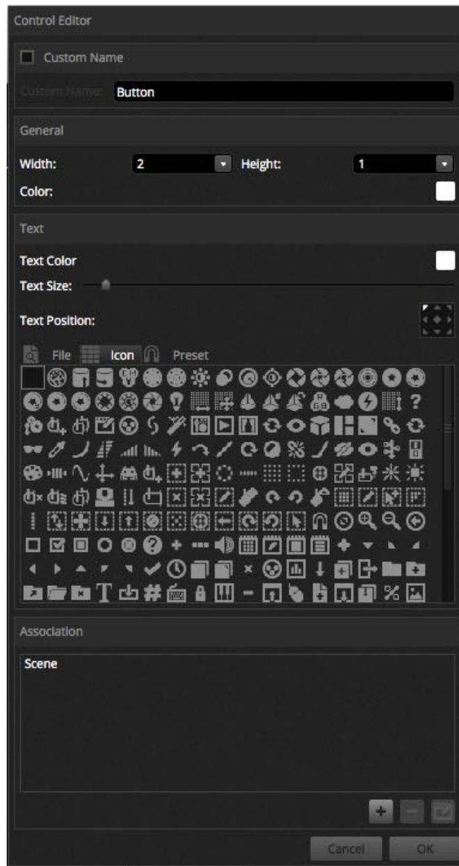
The association or pairing of a control can be edited by clicking 'Edit Association'. The Association window appears with a list of commands. Several commands may be added so that one button can be used to trigger several different scenes, or 1 fader can be used to control the speed of several scenes.
