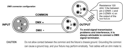
Cabling must have a male XLR connector on one end and a female XLR connector on the other end.
