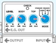
Boost the highs with the TOP control, and cut the lows with BODY. Perfect for getting a sound with fat mids and lows.
