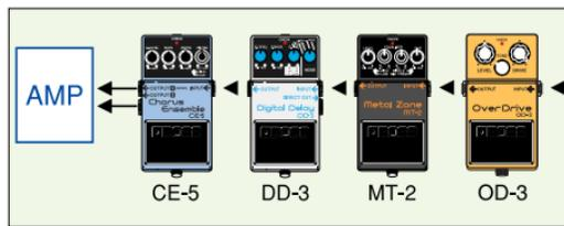
This setup provides a very versatile guitar sound. The OD-3 is used when you need a natural overdrive tone. The MT-2 is used when you need full-out thrash metal. Use the DD-3 as a doubler set at about 20ms. For chorusing add the versatile CE-5. Its filtering gives you a classic CE-2 warm chorus or a more contemporary sound depending on the settings.
