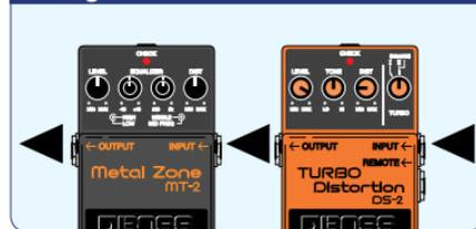
For an extreme distortion sound with earth-shaking results, plug into the DS-2 for a nice pre-boost and then plug into the MT-2 to take it over the top. To get a milder sound suitable for blues and rock solos, use the BD-2 or OD-3.
