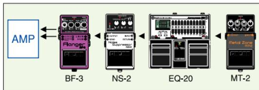
To get a monstrous seven-string metal sound, start with the MT-2 Metal Zone® and add the EQ-20 Programmable EQ on preset four to tighten up the low end. Use the NS-2 Noise Suppressor to wipe out any excess noise, and finish off with the BF-3 Flanger for some metallic icing on top.
