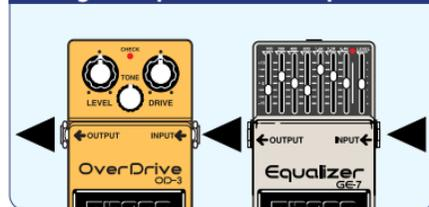
An equalizer and compressor can also be great boosters. Using the equalizer will raise gain as well as emphasize distortion over a specific frequency range. Using a compressor can also create a distinctive boost by varying tone and attack.
