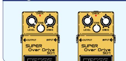
As the signal input to the amp increases, the distortion gets harder. Using an overdrive unit, raise the input signal gain. Here are two typical setups. Setting the amp for crunch gets the best results.
