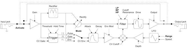
The input signal is first pre-amplified and then sent to the processing circuitry. This processing consists in a chain of three elements: Rectifier module - Multimode filter - Overdrive module.
