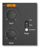
The 2-pole Filter is equipped with a low frequency oscillator (LFO) that can be used for cutoff modulation purposes. The LFO generates a periodic triangle waveform with adjustable frequency and depth.
