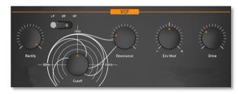
The 2-pole offers a multimode filter with rectifier and saturation. The signal path is: Rectifier -> Filter -> Saturation
