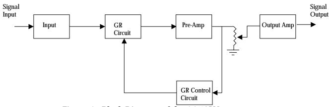
Figure 1 - Block Diagram of the 1176LN.
