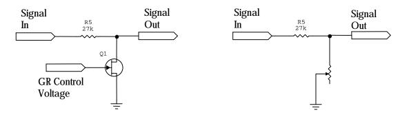
Figure 4 - Using a FET as a voltage-variable resistor. The combination of R5 and Q1 acts as a voltage divider which controls the gain.
