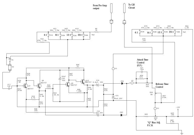
Figure 5 – 1176LN Gain Reduction Control Circuit.
