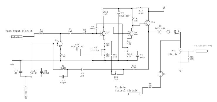
Figure 3 - 1176LN Gain Reduction stage.
