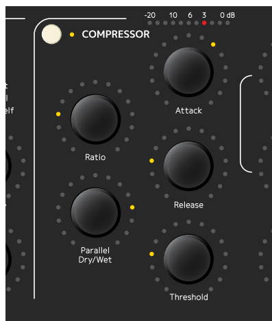
Compressor section on the Console 1 hardware.
