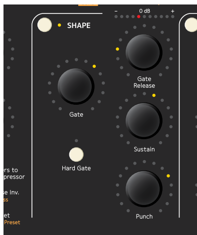
Shape section on the Console 1 hardware.
