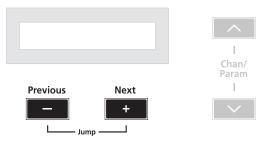
Pressing both **Next** and Previous **Value** buttons simultaneously will jump to the next category of items in the list. For example, when in Program Mode with program **1 Studio Grand** currently selected, pressing **Next** and **Previous** simultaneously will jump up the list of programs to program **8 Stevie's Rhds**, the first of the Electric Piano programs. Pressing the two buttons again will jump up to program **16 Supasticious**, the first of the Clavinet programs.
