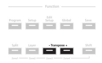
Pressing the **Transpose +** button will transpose the current Program up by one semitone; pressing the **Transpose –** button will transpose the current Program down by one semitone. Pressing both **Transpose +** and **Transpose –** simultaneously will restore the current Program to having no transposition; if these two buttons are simultaneously pressed when there is already no transposition, then the current Program will be transposed down by one octave (12 semitones).
