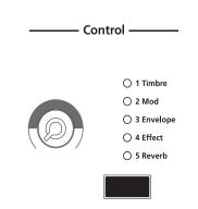
The control knob gives you real-time control of five different parameters—the currently selected parameter is indicated by the column of LEDs. By default these five parameters are:
