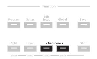
Pressing both **Transpose +** and **Transpose –** simultaneously will restore the current program or setup to having no transposition. If these two buttons are simultaneously pressed when there is already no transposition, then the current program or setup will be transposed down by one octave (12 semitones).
