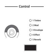
The control knob gives you real-time control of five different parameters—the currently selected parameter is indicated by the column of LEDs. By default these five parameters are:
