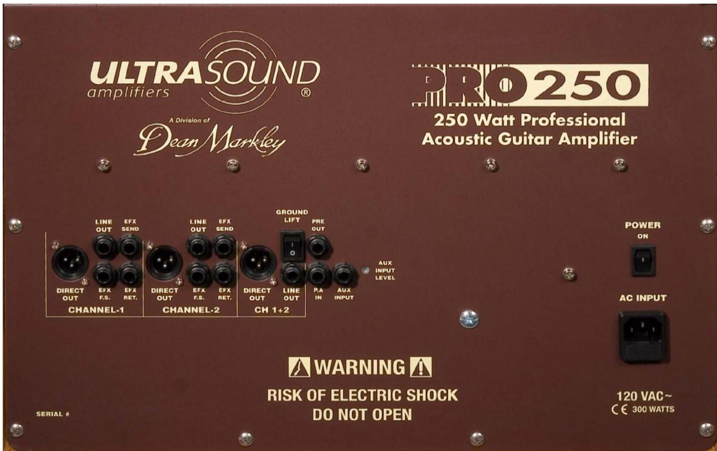
**DIRECT/LINE OUTPUTS:** The **PRO** has both XLR (balanced) **DIRECT OUT** and 1/4" (unbalanced) **LINE OUT** outputs. The XLR outputs can drive long cable lengths without added noise while the 1/4" outputs can drive virtually any line level input. Separate **CHANNEL-1**, **CHANNEL-2**, and **CHANNEL 1+2** outputs are post eq/efx to ensure a finished mixed signal to a PA system.
