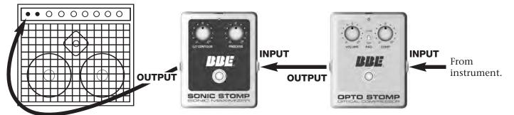
Connect the output of the first pedal to the input of the second pedal. Continue plugging outputs to inputs throughout the chain.
