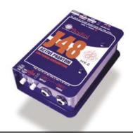
The Radial J48 direct box is the world's finest phantom-powered active DI. It has been optimized to handle extreme transients using only the 5 milliamps of available current from typical 48-Volt phantompower. The J48 features a unique digital switch-mode power supply that steps up the internal rail voltage to an amazing 9-Volts.
