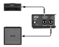
Connect the XLR output to a mic preamp input on your mixing console using a standard XLR microphone cable.
