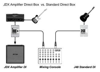
Bass and acoustic guitars often use a standard DI to capture the clean sound of the instrument. This works because these instruments almost always use an unprocessed sound and the PA system merely amplifies the levels of the direct signal.
