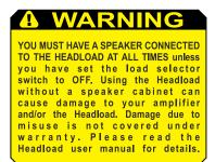
The danger is the LOAD switch could be bumped or moved and potentially put the Headload and/or amplifier at risk of damage. For this reason we recommend the Headload be connected to a speaker at all times. If you choose to ignore this warning, you should check the position of the LOAD switch before each use to minimize the risk
