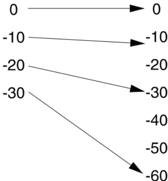
*As the input signal level decreases further below the threshold point, the output signal drops more rapidly.*
