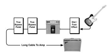
The PB1 should be placed ahead of any passive splits in the guitar signal such as "Y" cables or passive ABY amp switchers. Buffering the signal allows it to be split and sent to two or more devices, like a tuner and a couple of amps, without loading down the pickups. For example, the Radial BigShot ABY is a passive amp switcher that can split the signal three ways to feed two amps and a tuner as shown below.
