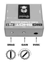
Connect the guitar to the PB1 input. Connect the output of the PB1 to the next device in the signal chain like an effect pedal or amplifier. Like many effect pedals, the PB1 may be powered by a standard 9V adaptor with a negative center conductor. The PB1 will be active the moment a 9VDC power supply is connected. There is no power switch and leaving the PB1 on for long periods of time will not cause damage.
