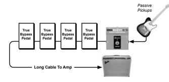
cables and jacks in your complex signal chain. Placing the PB1 directly after the guitar and before other pedals can restore the clarity and impact lost to capacitance.
